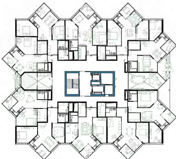
Grundriss 9.-21. Obergeschoss SAW 1:500
