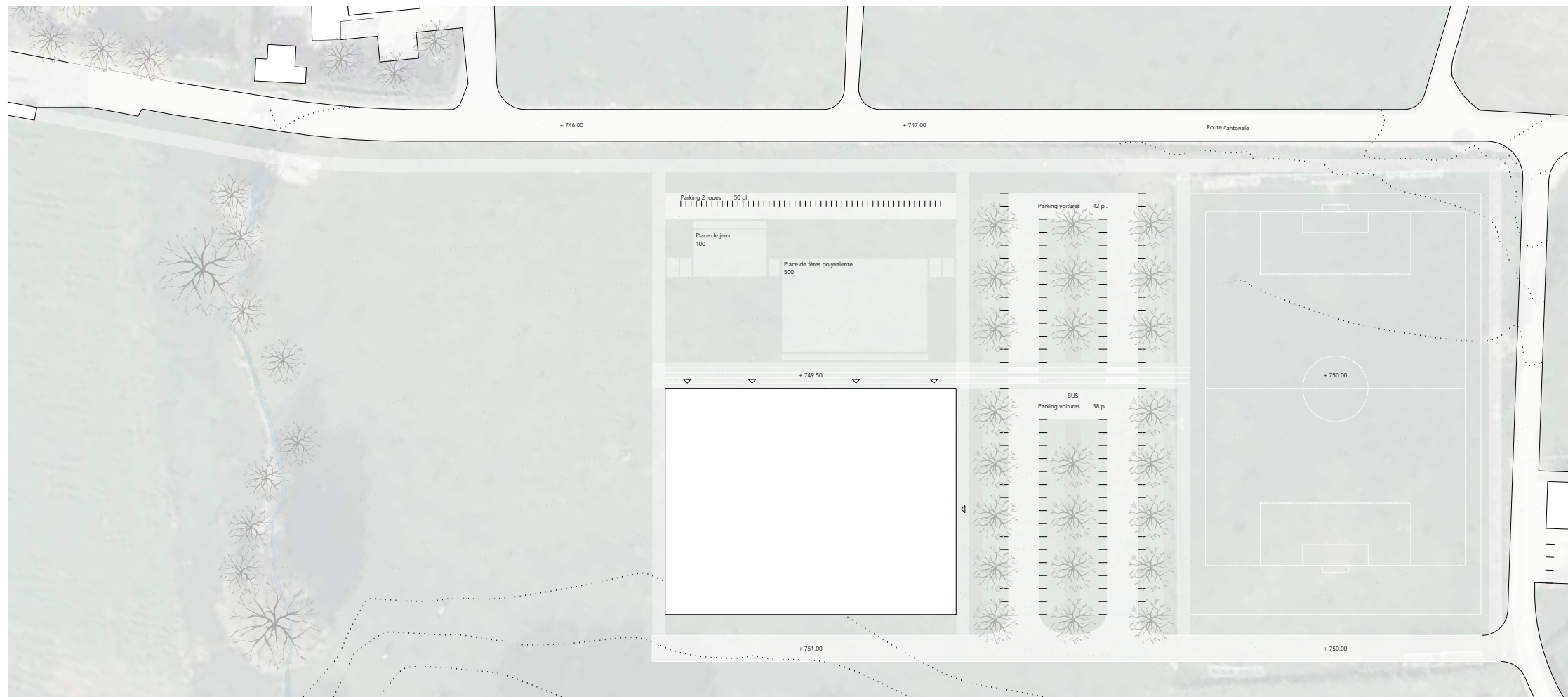
SITUATION 1:500 Surface de terrain (RF 398) = 16.066m 2 Surface routier = 1.662m 2 Surface de terrain déterminante = 14.404m 2 Surface bâti déterminante = 2.604m 2 Surface de plancher = 3.694m 2 IBUS = 0.26 IOS = 0.18 Solde de surface du plancher = 12.150m 2
