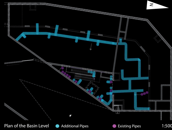
Plan of the Basin Level ● Additional Pipes ● Existing Pipes 1:500
